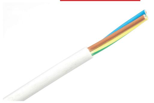
Made of Class 5 plain annealed copper conductors encased in a PVC-insulated sheath, this general-purpose flexible AC mains cable is used where the risk of mechanical damage and stress is within normal/minimal range. Ideal for everyday use of small to medium-sized equipment in domestic, commercial, and light industrial environments.
