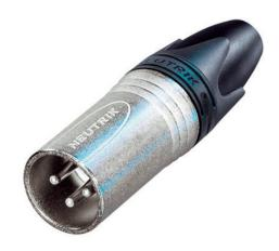
The Neutrik NC3MXX-HA is a 3 pole male cable connector with nickel housing, silver contacts and crimp termination (standard B crimp).
